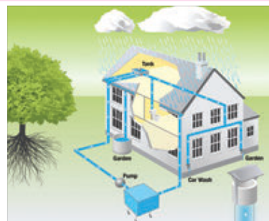
Fig. Rain water harvesting.
