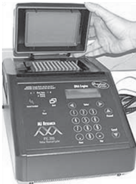
Fig.24.1: A PCR machine for the amplification of DNA.
